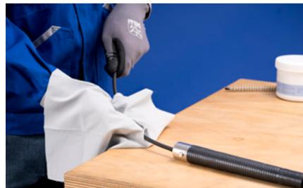
Degrease the core with a non-linting cleaning cloth.
