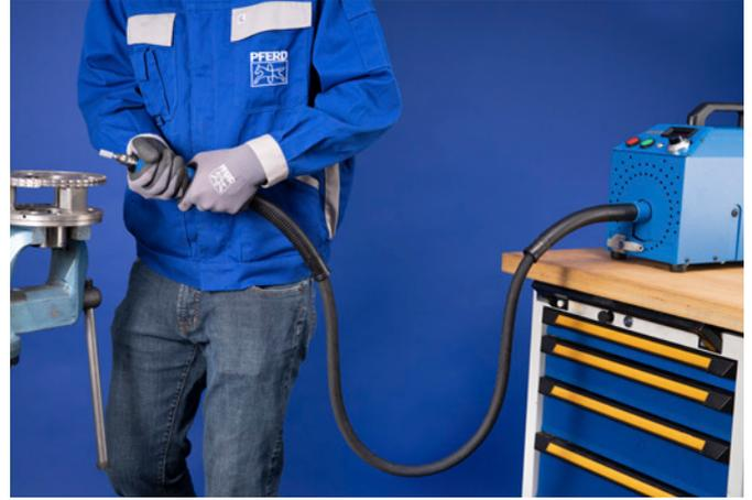
Flexible shaft drive set up incorrectly:
