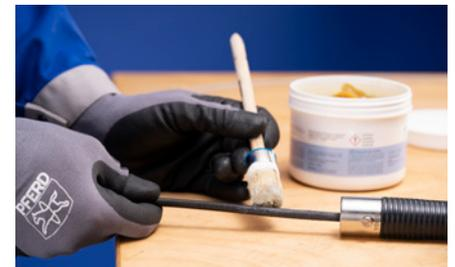
Then apply new special shaft grease to the core.
