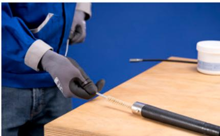
Clean the casing with the tube brush from the maintenance set.
