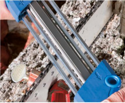
Chain saw sharpeners from PFERD are exceptionally well suited to the manual sharpening of saw chains. Manual sharpening is more economic and much more gentle than machine-based sharpening, and can prolong the operating life of the saw chain.
