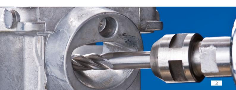
for use on aluminium/non-ferrous metals
