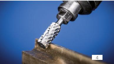
for use on aluminium/non-ferrous metals
