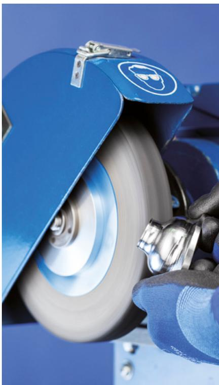
POLINOX non-woven tools PNK consist of spiral-shaped, non-woven abrasive which is wound around a core and foamed up. The foam supports the non-woven component and positively impacts its tool life and abrasive performance. This particular bond results in non-woven wheels with a very good surface finish, high stock removal rate and long tool life.
