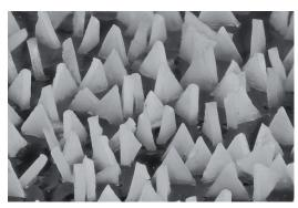
Of course most users value the enormous power of the triangular, precision-moulded high performance abrasive. "**VICTO**GRAIN outperforms other, established solutions by up to 30% – with a consistent degree of aggressiveness," said Heimann. It performs impressively in use. While other abrasives offer a similarly high level of aggressiveness at the beginning of use, it usually
